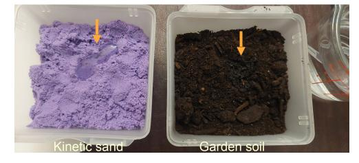
Result 3 Water Absorption Test.
